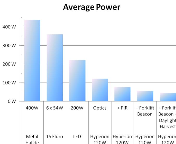
The system is also failsafe and can be retrofitted at a later date. This is because the lights operating independently of the Proximity Beacons. If the beacons are turned off, the system reverts back to its basic operating mode (which might include daylight harvesting and PIR proximity functions).
